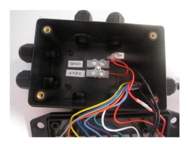
Fit the bottom again and check that the cables are not trapped. Fasten the four screws again.
