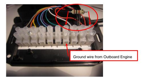
Input #1 which is now used as Outboard Engine alarm is activated in the app. As shown below.
