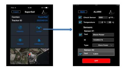
In the above example, we have decided to activate the Shore Power Sensor as sensor #1, but all sensors are available for all sensor types.
