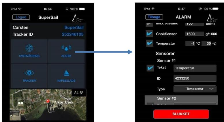
In the above example, we have decided to activate the Temperature sensor as sensor #1, but all sensors are available for all sensor types.
