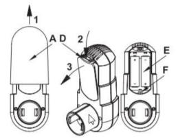
Insert the batteries into the battery cabinet ensuring proper polarity (see polarity marks).
