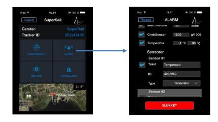
In the above example, we have decided to activate the Humidity/Temperature sensor as sensor #1, but all sensors are available for all sensor types.
