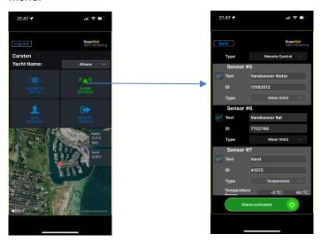
In the above example we have activated a water sensor as sensor #5 and #6 – several water sensors can be connected, and all wireless sensor fields can be used.
