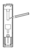
Press and hold the button for 5 seconds, until the LED starts blinking slowly with red light (use a tip pen).
