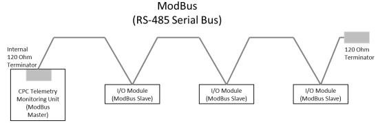
**Note:** RS-485 serial communications uses a voltage differential signal, that requires proper termination with a 120 Ohm resistor in both ends of the network cable. This follows RS-485 standard for biasing to ensure reliable performance
